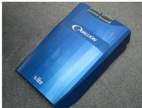
Quallion X-51A Lithium-Ion Battery.
