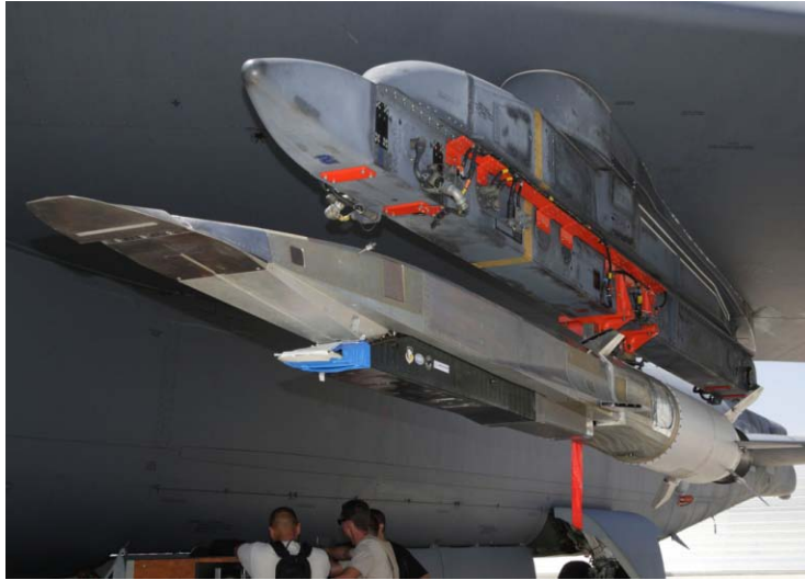
X-51A during B-52 Fit Check.
